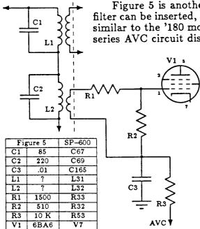
Figure 5 is another part of a SP-600 schematic where a mechanical filter can be inserted, and Figure 6 below shows the modification which is similar to the '180 modification in Figure 2. Figure 6 also illustrates the series AVC circuit discussed in Part 2 (HSN 12). It requires a bit more
