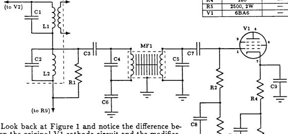
Look back at Figure 1 and notice the difference between the original V1 cathode circuit and the modification in Figure 2. All mechanical filters introduce some signal loss, called insertion loss, typically on the order of 6 - 8 db or about 1 S-unit. Insertion loss is usually
