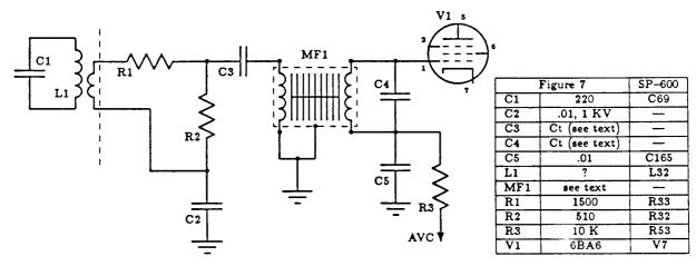
As I said above, for the SP-600 there is a simple way to compensate for any reasonable (5-10 dB) insertion loss introduced by a mechanical filter. Figure 8 shows the method: unsolder the wire at the junction of R1 (R95) and R2 (R96), remove R2 (R96), and replace it with a 25 K, 2 W variable. The R1-R2 circuit is a voltage divider which provides
